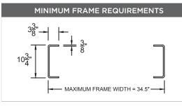
Minimum section modulus per rail = 17.8 in.<sup>3</sup> Minimum yield strength = 110 KSI
